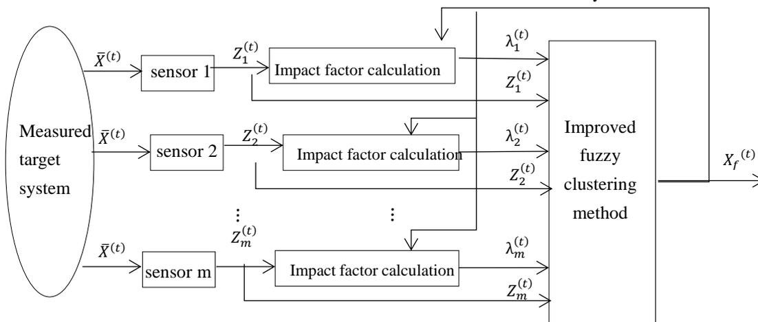
Figure 2. Structure of the data fusion method based on advanced fuzzy clustering
